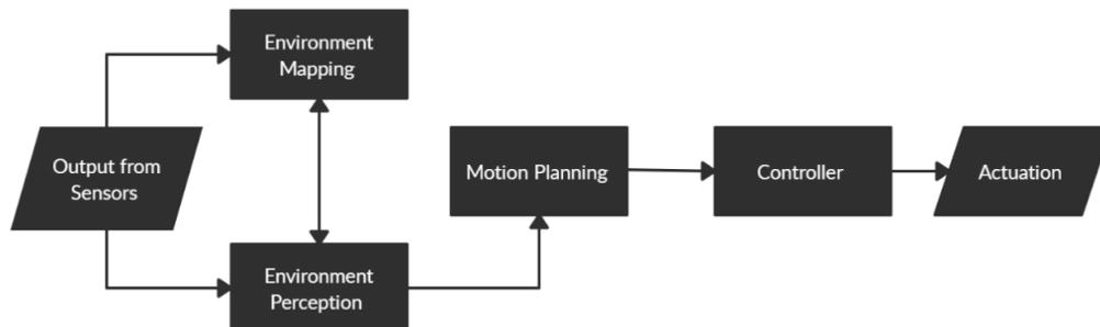
Figure 1. Architecture of a self-driving vehicle.
